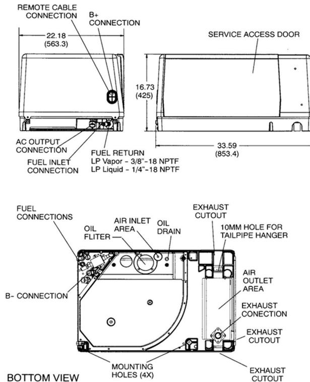
**Note:** This outline drawing is provided for general reference only and is not intended for design or installation. For more information see Operation and Installation manuals or obtain drawing 500-3234 and wiring diagram from your distributor/dealer.
